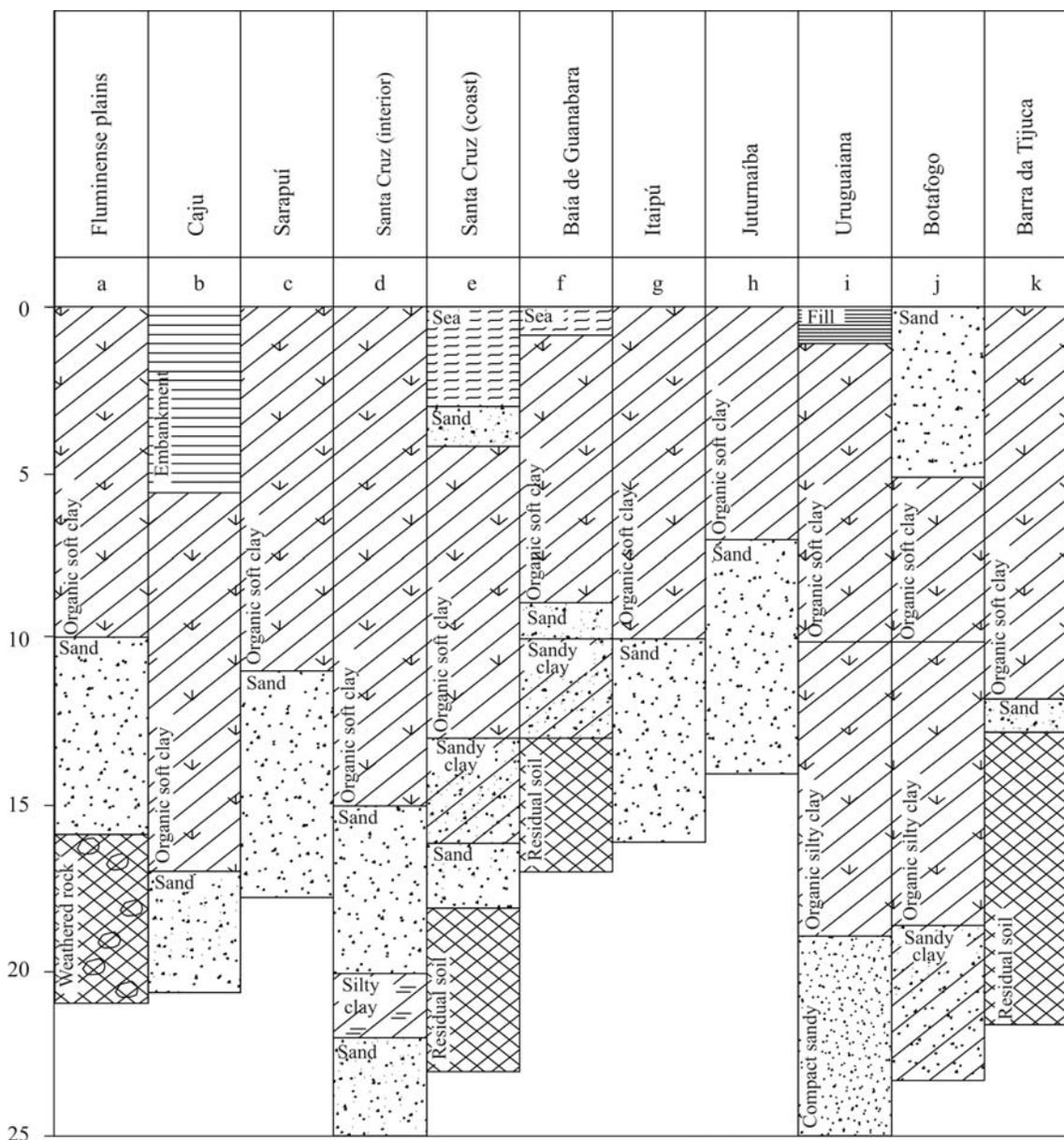
**Figure 1** - Geotechnical profiles of Rio de Janeiro clays.
