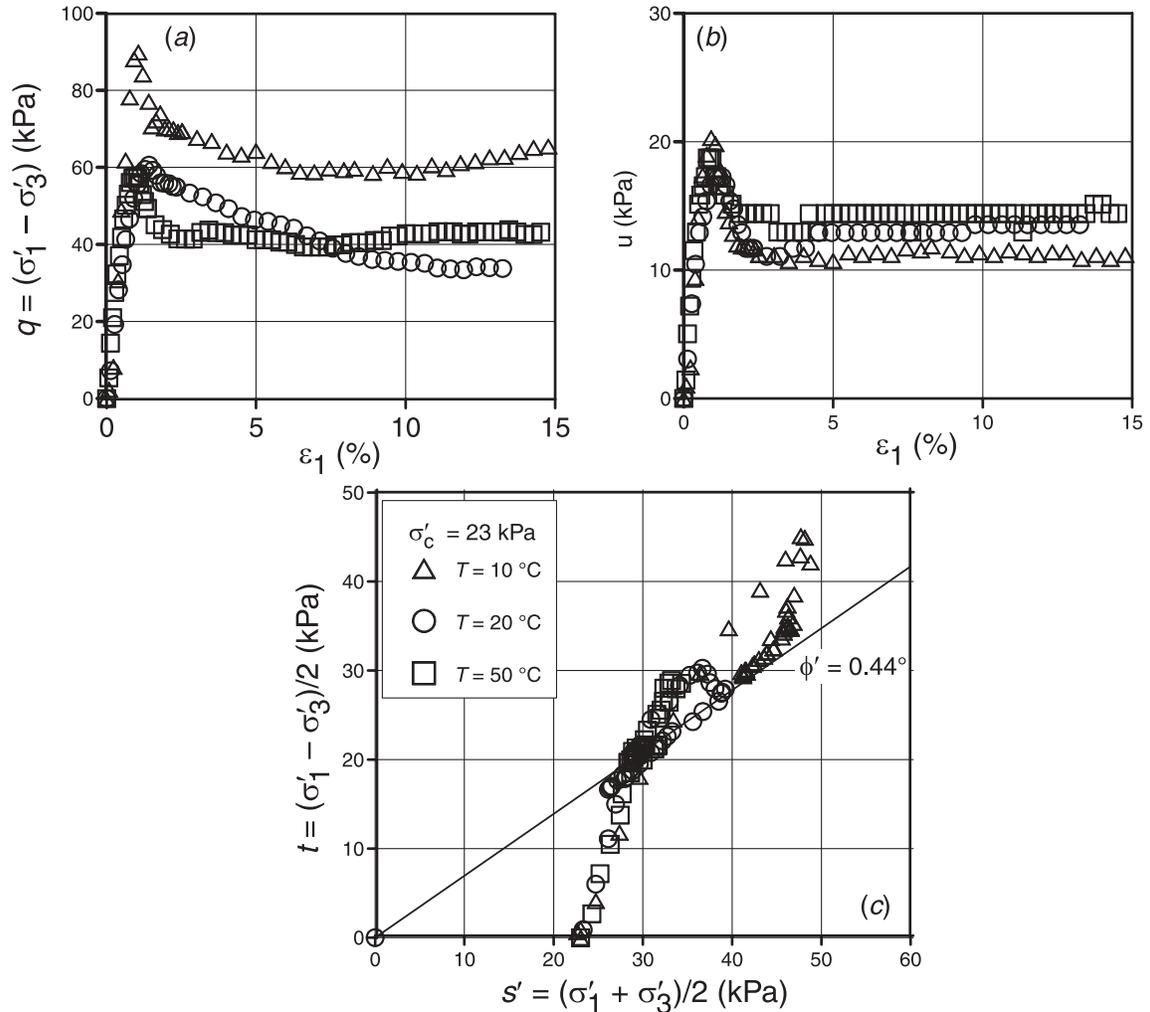
**Fig. 11.** CIU tests results in the normally consolidated range ( $T = 10\text{--}50\text{ }^\circ\text{C}$ ): (a) compression curve; (b) stress ( $q$ ) – strain and pore pressure – strain curves; (c) stress path.
