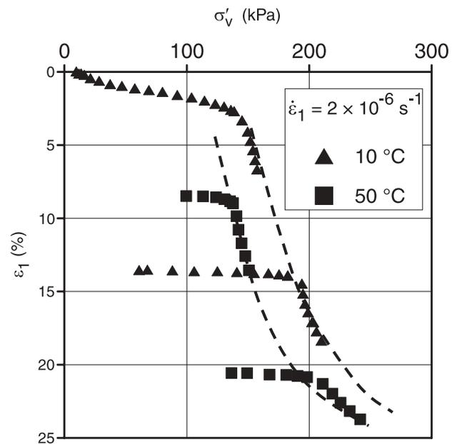
Figure 5b shows the same vertical yield stresses obtained at different strain rates as a function of temperature. The curves are in relatively good agreement with the following relationship proposed by Moritz (1995):
