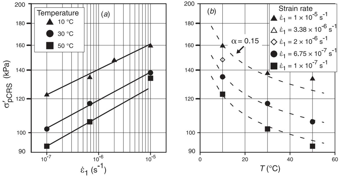
Fig. 6. Normalized viscosity and vertical yield stresses for clays of different origins, as a function of temperature.
