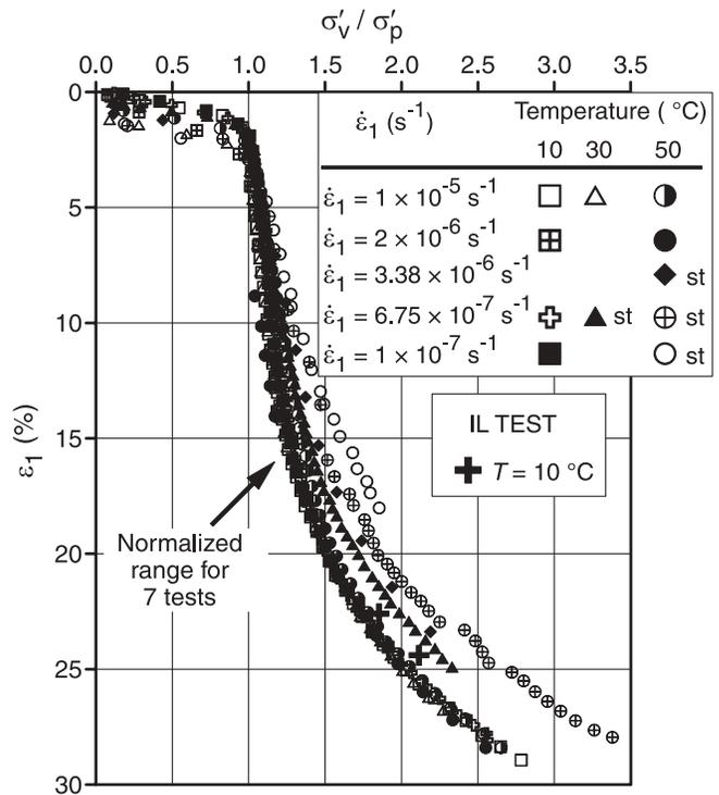
140 kPa, in excess of the vertical yield stress of the clay (Fig. 19a). The specimen was then heated to 20, 35, and 50 °C in steps with duration of at least 48 h. The specimen
