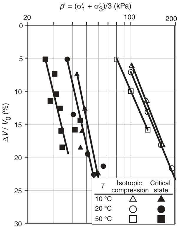
Fig. 16. Schematic variation of limit state surface with strain rate or temperature.
