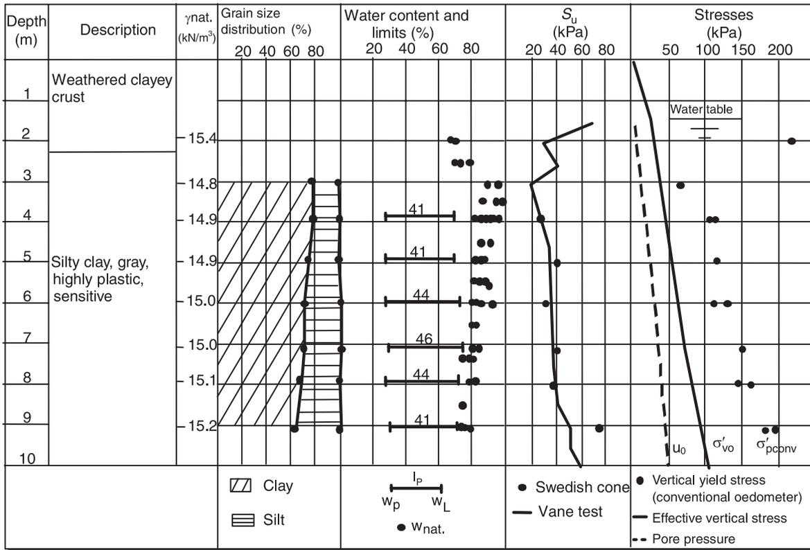
Fig. 2. Variation of vertical yield stresses and in situ vertical effective stress with depth for St-Roch-de-l’Achigan clay.
