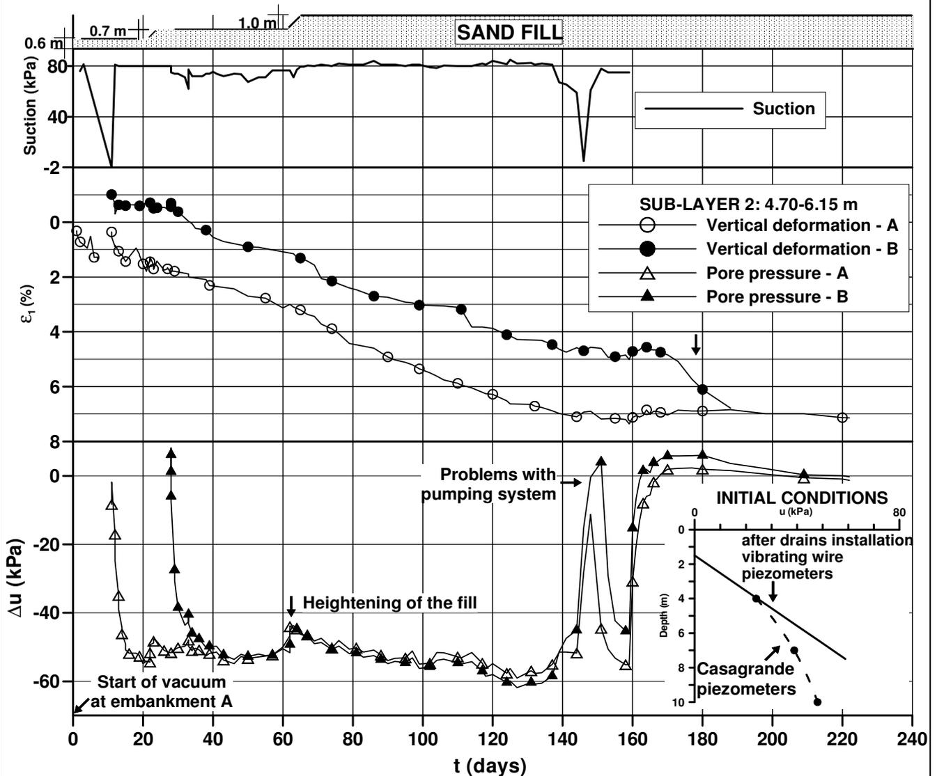
Figure 6. Suction, vertical deformation and pore pressure variation with time at sub-layer 2.
