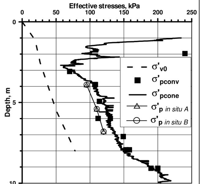
Figure 9. Vertical yield stress and *in situ* vertical effective stress profiles.
