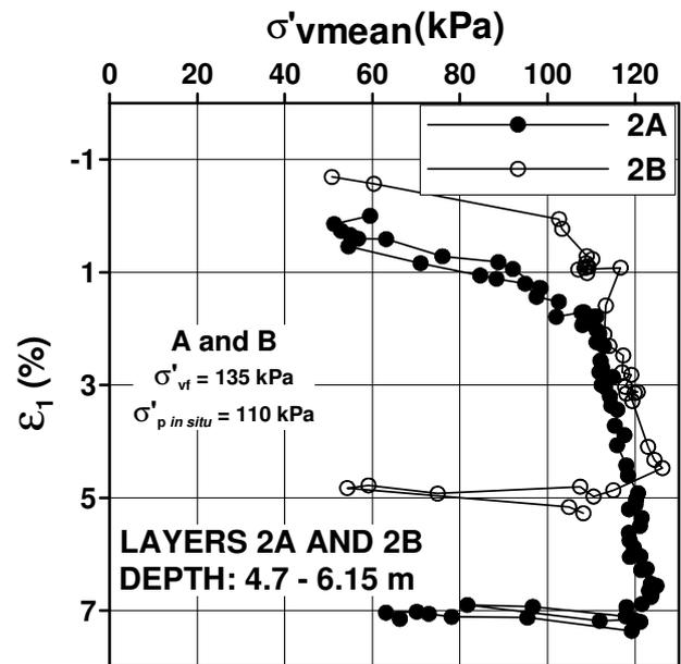
Figure 8. Compression curve of sub-layers 2A (fill A) and 2B (fill B).
