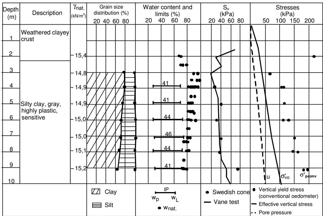
Figure 2. Geotechnical characteristics of Saint-Roch-de-l'Achigan clay deposit (Marques et al. 2000).
