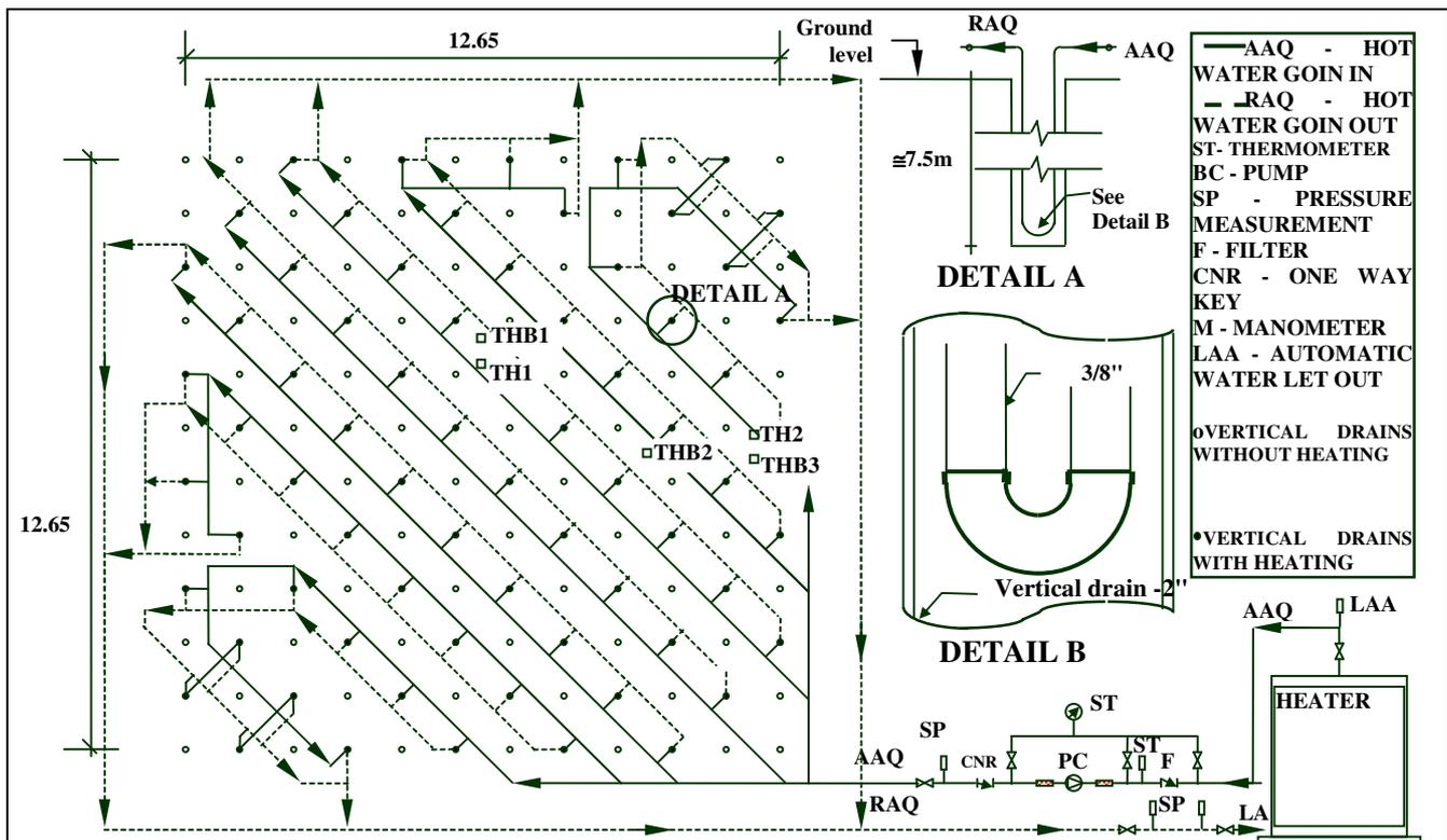
Figure 3. Layout of the heating system.
