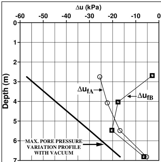
Figure 7. Pore-pressure profiles at the end of pumping.
